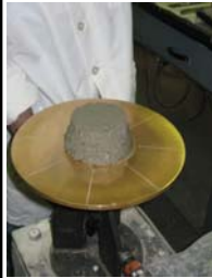
6. Lift Mold 1 Minute after Mixing.
