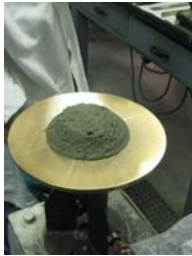
7. Immediately Drop the Table 25 times in 15s.
