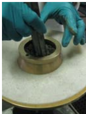
2. Tamp 20 Times. Incline Tamper when Near Perimeter.
